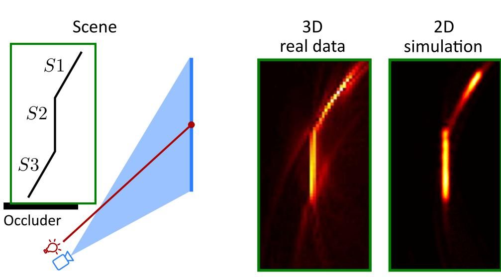
We validate our system by replicating previous works [3] in our 2D simulation system. Known visibility problems remain and prevent us from reconstructing S3.
