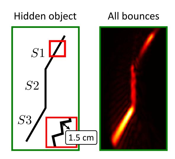
We use our system to further analyze visibility and change the local structure of the object. In the presence of facets, we can image S3.
