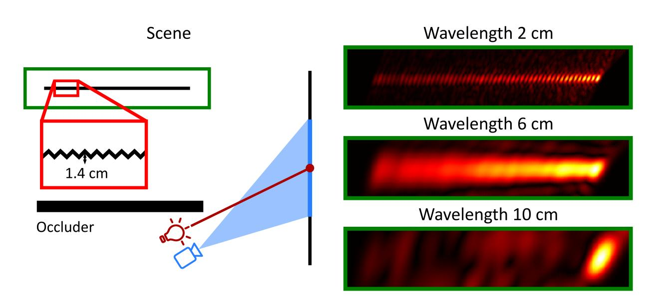
We explore the effect of filtering with different central wavelengths to reproduce local features on a globally planar object. Depending on the relationship between feature size and the chosen wavelength, we reconstruct the object with different levels of detail.
