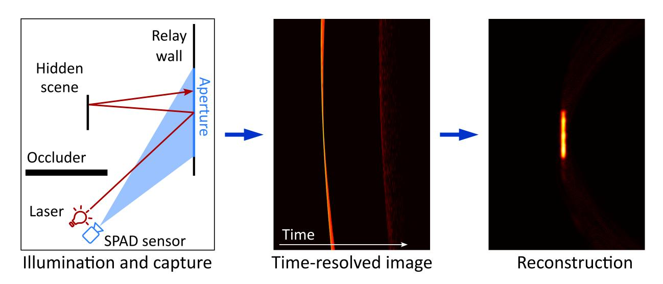
An ultra-fast laser pulse illuminates the relay wall and scatters towards the hidden scene. A SPAD-based sensor captures time-resolved indirect illumination at the relay wall. Based on the time of flight of third-bounce light paths, we reconstruct the hidden scene.
