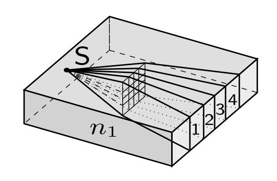
depicting Illustration the field of view (FoV) ToF the sensor optical within an waveguide.
