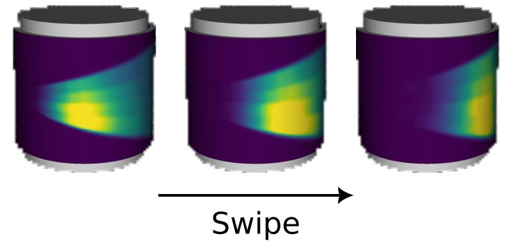
Real OptoSkin prototype fabricated using a rigid waveguide realized with 3D printed material (CrystalClear ring of Monocure3D). We show the reconstruction of swipe.
