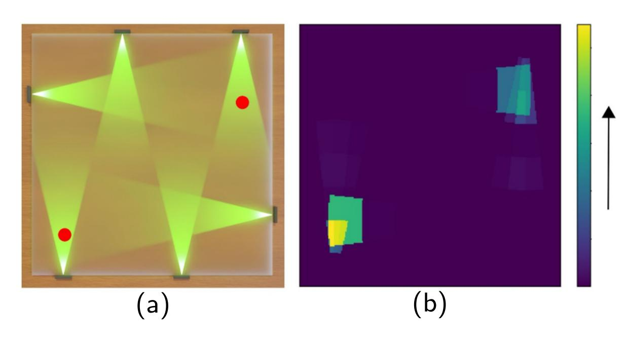
(a) A digital twin of the OptoSkin setup with six ToF sensors and two touches on the red circles. (b) We simulate light transport inside the waveguide. From the simulated ToF signal, we reconstruct the two touch locations by triangulating the ToF of the light
